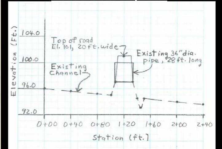
**Slide 5.** This is a plot of the field survey notes shown in the previous slide. Seeing a graphical representation of the stream channel, road and pipe help to determine the proper elevation the replacement culvert should be located and how long the pipe should be.
