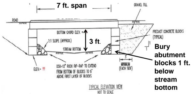
**Slide 16.** Another alternative is to use an open bottom bridge. The bridge option has the flexibility of multiple widths and heights and can be a cost effective option if one lane traffic is adequate. Bridges are a good option to use for sites that have a relatively low road fill. Using a bridge at low road fill sites will require abutments of a reasonable height and not require so much extra road fill that a culvert may require.
