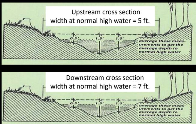
**Slide 3.** Two typical cross sections should be obtained in order to insure the pipe is sized correctly. Two typical cross sections are shown in this example, one upstream and one downstream.
