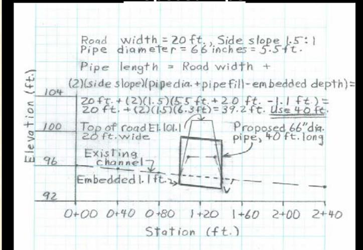
**Slide 10.** This slide shows a plot of the proposed pipe in relation to stream channel and road cross section. Note how much the bottom of the pipe has been lowered compared to existing 36 inch pipe. The proposed pipe is embedded 20% below the estimated original channel bottom under the road. The calculations show how the pipe length is determined taking into account the road top width, pipe diameter, and stable side slopes for the road shoulders (typically 1.5:1 or flatter).
