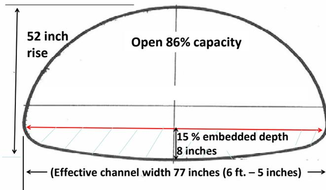
**Slide 14.** This slide shows a cross section of the full bottom invert pipe arch option. This is a better approach for a “stream smart” crossing as the effective channel width of the structure exceeds the average channel width. Again adding channel substrate material is preferable especially for wider flatter openings to insure a low flow channel forms for better fish passage at low flows.
